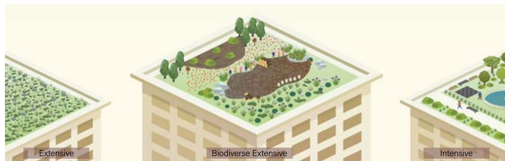
Figure 7.1: Types of greenroofs
