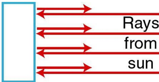
A flat face of a building or other structure reflects the sun but does not focus or concentrate it.
