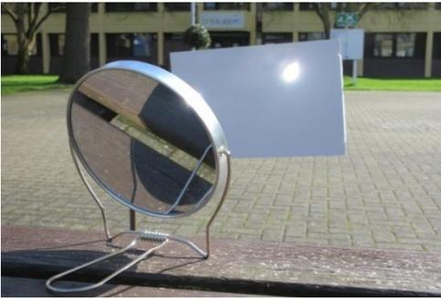
The photograph shows a concave mirror focussing the sun's rays. Focussing of the sun can also happen in buildings, with the old-fashioned 'bulls-eye' types of glass. However in this case the sun is focused inside the building, not outside.
